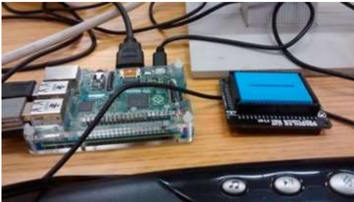
On the left, a Pi running a QL emulator and a Propeller development hat for the Pi
